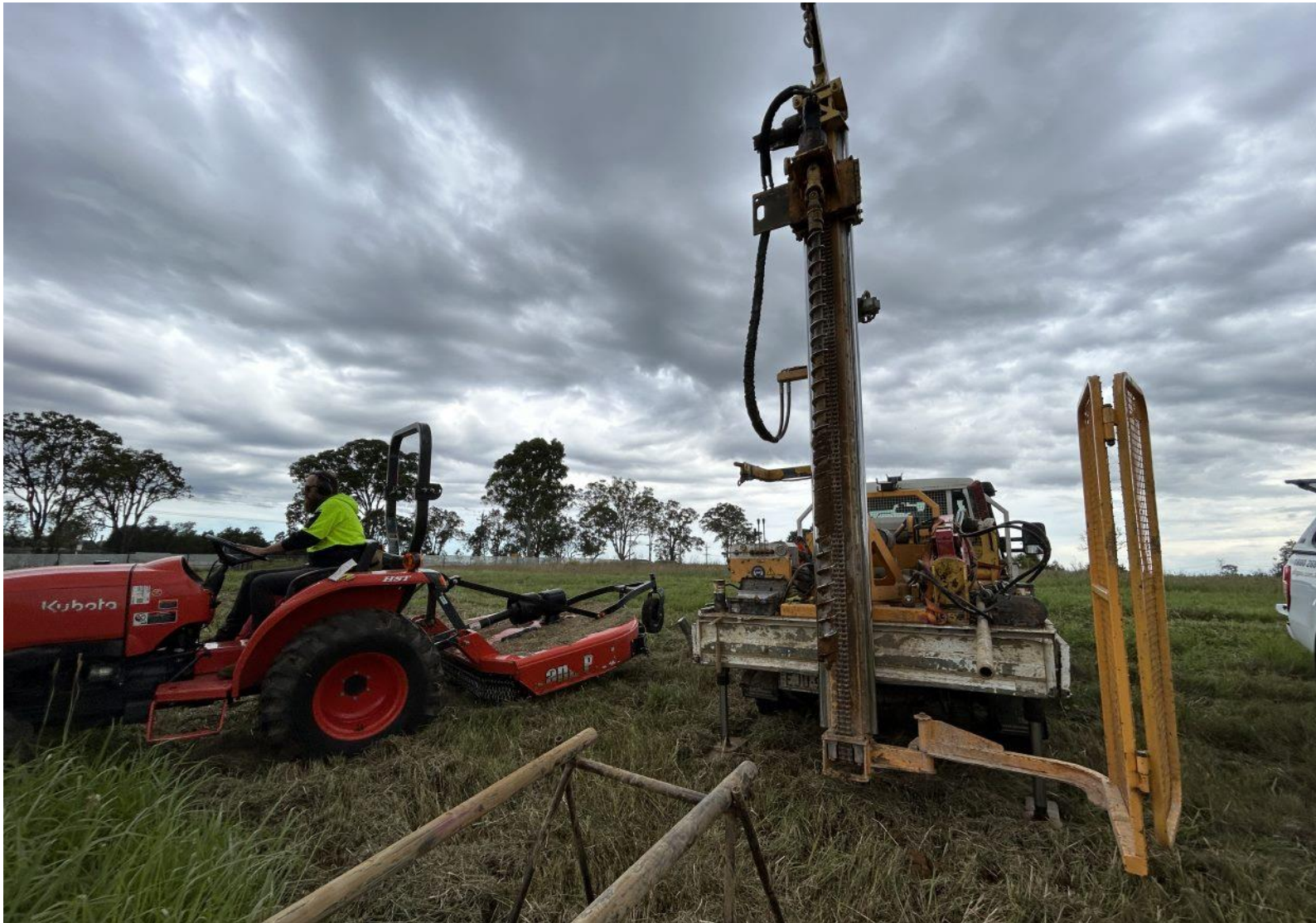
Photo 2 - Borehole BH01 drilling rig setup
